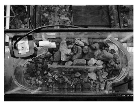
FIGURE 1.—Top view of aquarium modified to simulate pulsed, high-velocity water (>35 cm/s) and stable, low-velocity water (<10 cm/s). Water pumps were placed in squared pockets to prevent the eggs and larvae from being sucked into the water intakes.
